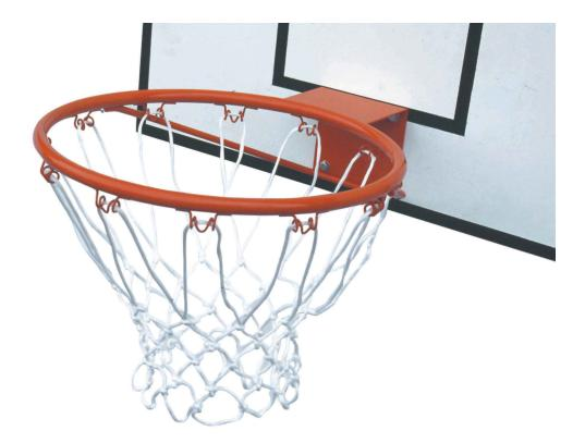
Regulation basket in orange painted steel, ring diam.mm.20x1,5 thickness, plate with thickness mm.3 and width mm.150 x150, 12 hooks diam.3mm, tie rod diam. 10 mm.
