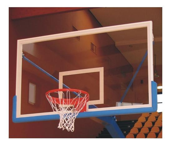
Glass backboard thickness mm. 12 with frame. Tempered glass with safety film to avoid falling fragments in case of breakage, dimensions cm.180x105, Withdrawal that allows the basket to be hooked directly onto the frame. Frame in white painted steel.
