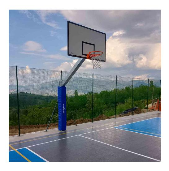
Structure in hot galvanized steel section cm. 15x15, extension cm. 225, complete with ground steel painted sockets, wooden regulatory backboards cm.180x105 in white / black color painted, support steel frame for backboards, baskets and nets regulamentary, uprights are supplied disassembled to facilitate assembly and transport. UNI EN 1270 certificate
