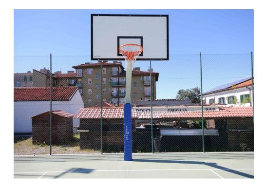
Structure in hot galvanized steel section cm. 15x15, extension cm. 165, complete with ground steel painted sockets, wooden regulatory backboards cm.180x105 in white / black color painted, support steel frame for backboards, baskets and nets regulamentary, uprights are supplied disassembled to facilitate assembly and transport. UNI EN 1270 certified plant. Two complete stations.
