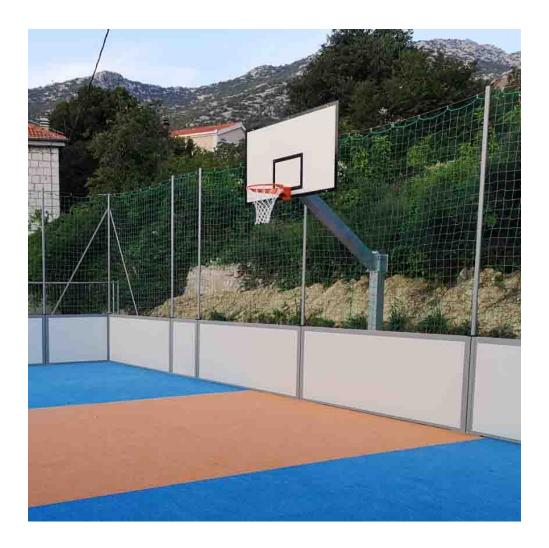
Hot-dip galvanized steel tubular structure section cm. 15x15, **overhang cm. 225**, complete with painted steel bushings to be planted, **regulation melamine resin backboards 180x105 cm.**white/black silk-screened, hot-galvanized steel backboard support frame, regulation baskets and nets.
