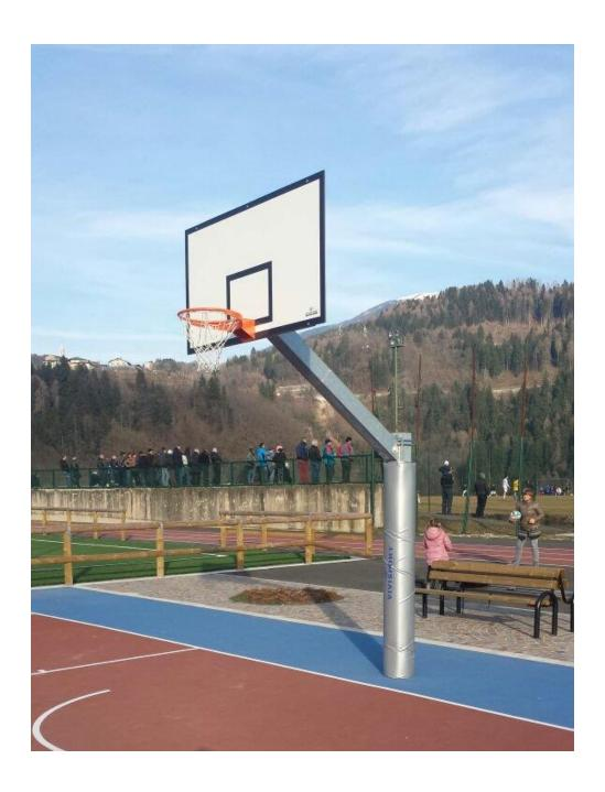
Hot-dip galvanized steel tubular structure section cm. 15x15, **overhang cm. 225**, complete with painted steel bushings to be buried, **regulation wooden backboards cm.180x105** silk-screened in white/black, backboard support frame in galvanized steel, baskets and regulation nets.
