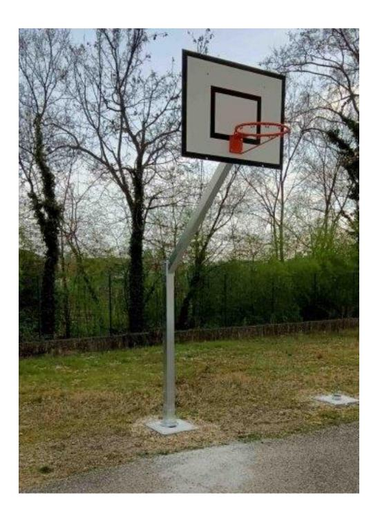
Hot galvanized tubular steel structure section cm. 10x10, overhang 120 cm, fixing with plate, 120x90 cm screen-printed melamine resin backboards in white / black, backboard support frame in galvanized steel, standard baskets and nets. All components are supplied disassembled to facilitate transport, during assembly you can choose the desired playing height minibasket / basket.
