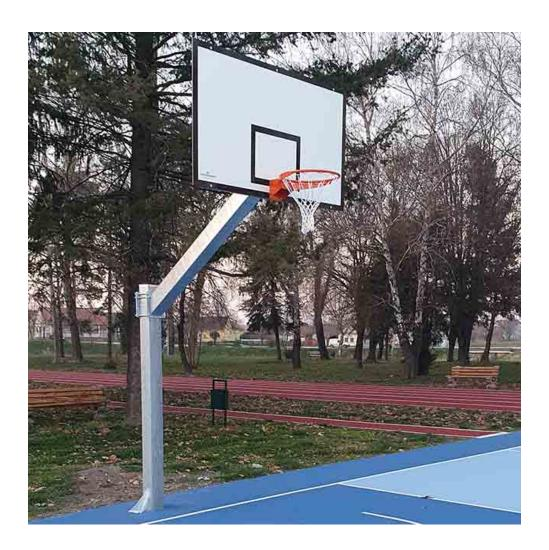
Single-tube basketball system**with wooden backboards**, hot-dip galvanized steel tubular structure, section cm. 15x15, **overhang cm.165**, complete with painted steel bushings to be planted, **regulation backboards cm.180x105** screen-printed in white/black, backboard support frame in hot-dip galvanized steel, baskets and regulation nets.
