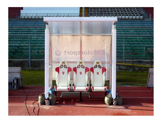
Team shelter model "Strong Plus" 1 m. long (2 seats), in aluminium, front struts construction mm. 60x70, cell-like policarbonate panels thickness mm. 4, seats in polypropylene.
