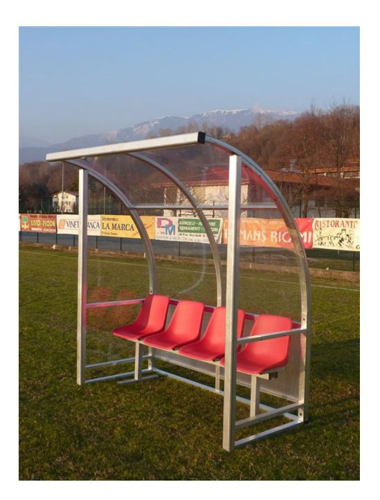
Bench model "Strong" 6 meters (12 seats), covers and sides made entirely of aluminum with 60x70 mm oversized front safety uprights. Semi-transparent honeycomb polycarbonate cover 4 mm thick. Seat frame in hot-dip galvanized steel and polypropylene shells with back.
