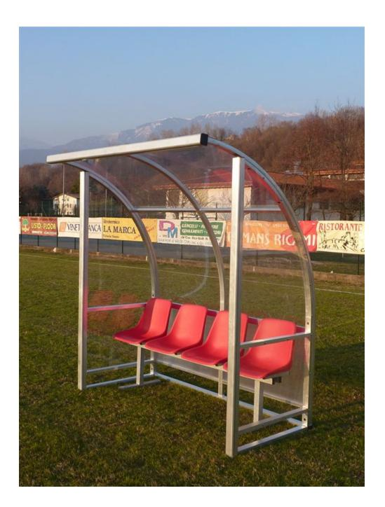
Bench model "Strong" 3 meters (6 seats), covers and sides made entirely of aluminum with 60x70 mm oversized front safety uprights. Semi-transparent honeycomb polycarbonate cover 4 mm thick. Seat frame in hot-dip galvanized steel and polypropylene shells with back. **Dimensions:**
