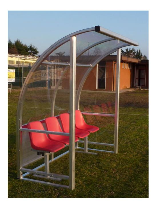
Bench model "Strong" 4 meters (8 seats), covers and sides made entirely of aluminum with 60x70 mm oversized front safety uprights. Semi-transparent honeycomb polycarbonate cover 4 mm thick. Seat frame in hot-dip galvanized steel and polypropylene shells with back. **Dimensions:**
