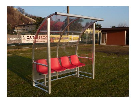
Bench model "Strong" 2 meters (4 places), covers and sides made entirely of aluminum with 60x70 mm oversized front safety uprights. Cover in 3 mm thick transparent compact polycarbonate. Seat frame in hot galvanized steel and polypropylene shells with back. **Dimensions:**
