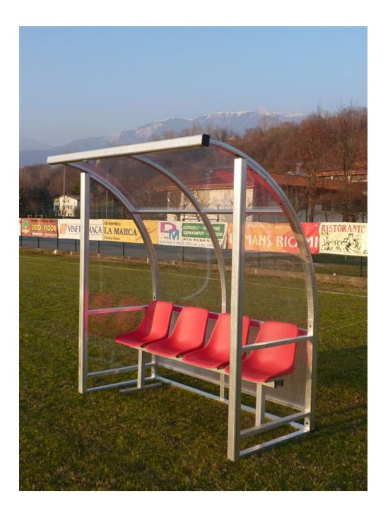
Bench model "Strong" 4 meters (8 seats), covers and sides made entirely of aluminum with 60x70 mm oversized front safety uprights. Cover in 3 mm thick transparent compact polycarbonate. Seat frame in hot galvanized steel and polypropylene shells with back.
