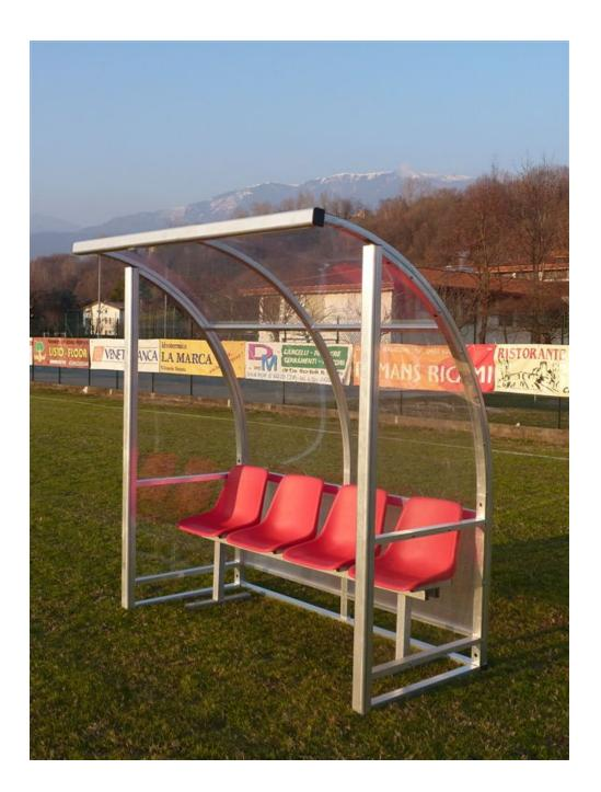
Bench model "Strong" 3 meters (6 seats), covers and sides made entirely of aluminum with 60x70 mm oversized front safety uprights. Compact transparent polycarbonate cover 3 mm thick. Seat frame in hot galvanized steel and polypropylene shells with back.
