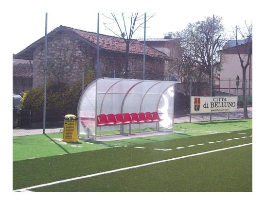
Team shelter model "Standard" 5 m. long (10 seats), in galvanized steel, cell-like policarbonate panels thickness mm. 4, seats in polypropylene.
