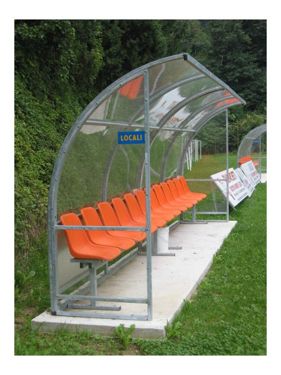
Bench model "Standard" 1 meter (2 places) covers and sides made of hot galvanized steel section 50x30 mm. Cover in compact transparent polycarbonate 3 mm thick. Seat frame in hot-dip galvanized steel and polypropylene shells with back.
