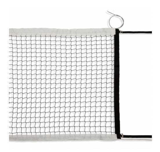
Volleyball net in high tenacity polyester, UV stabilized, worked without knot. Upper band in PVC 70 mm with double stitching and steel cable Ø 5 mm. Lower band in PVC 50 mm with double stitching and polyester rope Ø 6 mm. On the sides finish with black band and fiberglass rod Ø 10 mm to facilitate traction. Complete with mobile antenna holder bands (excluding antennas). Ability to print on ribbons, even in multiple colors.
