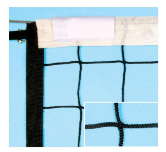
Volleyball net, in high tenacity polyester, UV stabilized, thermofixed, worked without knot. 100x100mm mesh Upper band in polyester 70 mm stitched and steel cable Ø 5 mm. Lower band in polyester 50 mm stitched and polyester rope Ø 6 mm. Black band on the sides with round fiberglass insert Ø 10 mm for traction. Mobile bands for antennas included. Product compliant with FIVB regulations. Network compliant with EN 1271: 2004.
