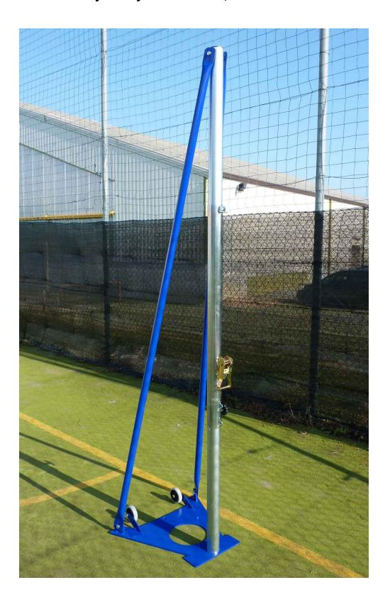
Trellis system for tennis use competition model. Structure composed of central upright in round tube diam. 70 mm. in galvanized steel, anchored on a large support plate with holes for fixing to the ground using dowels. Tubular steel tie rods diam. 40mm., Equipped with wheels for transport. Network height adjustment using galvanized slides. Complete with tendirete.
