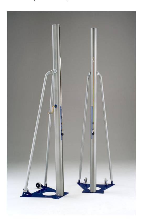
Trellis volleyball system with aluminum tie rods with reduced dimensions mod. "All Aluminum" built entirely in aluminum alloy, new reinforced section to give more stability and strength to the system. Steel tie rods with reduced overall dimensions. Anti-torsion ground fixing plate in laser-cut steel, innovative self-braking net tensioner winch
