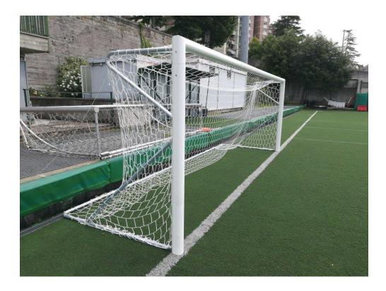
Pair of 5x2 meters divided crossbar goals, mobile, made with 100x120 mm oval section aluminum profile. with internal profiles. To make the goal even more stable and sturdy, the elbows are welded and the joints are in high-thickness profile in special alloy 6005 aluminum. Elbow in hot-galvanized steel and plastic hooks for fixing the net. Flap protection art. 6040 not included
