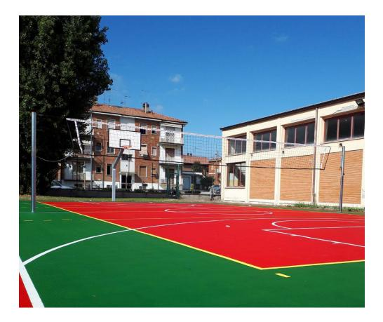
Monotubolar volleyball system in galvanized steel diam. 100 mm. complete with net tensioner, fixing to the floor by means of bushings to be cemented. Network height adjustment system by means of galvanized steel slides. Complete with bushes and caps.
