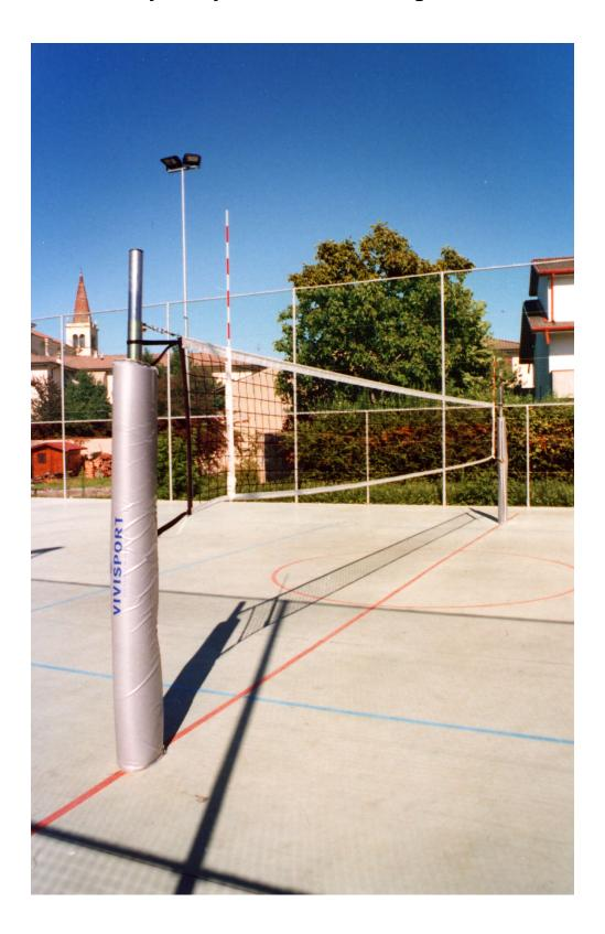
Monotubolar volleyball system in galvanized steel diam. 70 mm. complete with net tensioner, fixing to the floor by means of bushings to be cemented. Network height adjustment system by means of galvanized steel slides. Complete with bushes and caps.
