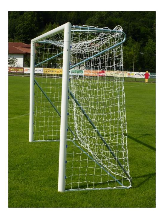
Pair of freestanding soccer goals 4x2 meters, made in aluminum profiles round section diam. 80 mm. with internal ribs. To make the goal even more stable and robust elbows are welded and the junctions are made with high thickness profile. Net support and ground frame made in galvanized steel, plastic hooks for securing the net.
