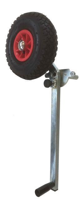
Football goal moving system mod. UNI standards, the kit includes 4 devices that can be operated manually, by means of a spring piston with 3 positions and a knob to facilitate its use. anti-mud rubber wheels, which allow movement in the various fields. specify when ordering where the kit must be applied.
