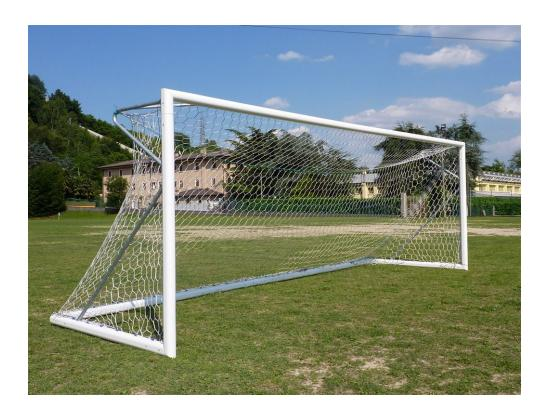
Pair of freestanding soccer goals 7.32x2.44 meters UNI-EN 748 tested, made in aluminum profiles oval section 100x120 mm. with internal ribs. To make the goal even more stable and robust elbows are welded and the junctions are made with high thickness profile in special aluminum alloy 6005. Curved net support made in hot galvanized steel, plastic hooks for securing the network.
