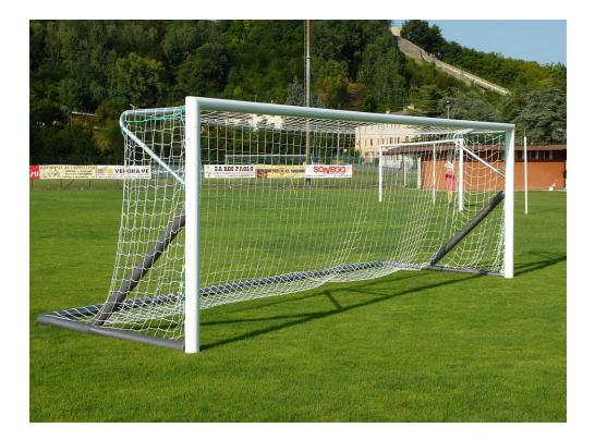
Pair of freestanding soccer goals 6x2 meters, made in aluminum profiles oval section 100x120 mm. with internal ribs. To make the goal even more stable and robust elbows are welded and the junctions are made with high thickness profile in special aluminum alloy 6005. Net support and ground frame made in hot galvanized steel, plastic hooks for securing the net.
